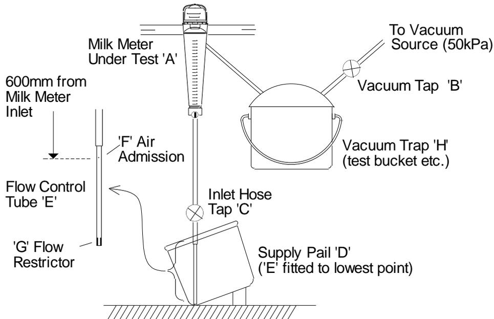
Fig 11.1 Basic Milk Meter Test Rig
